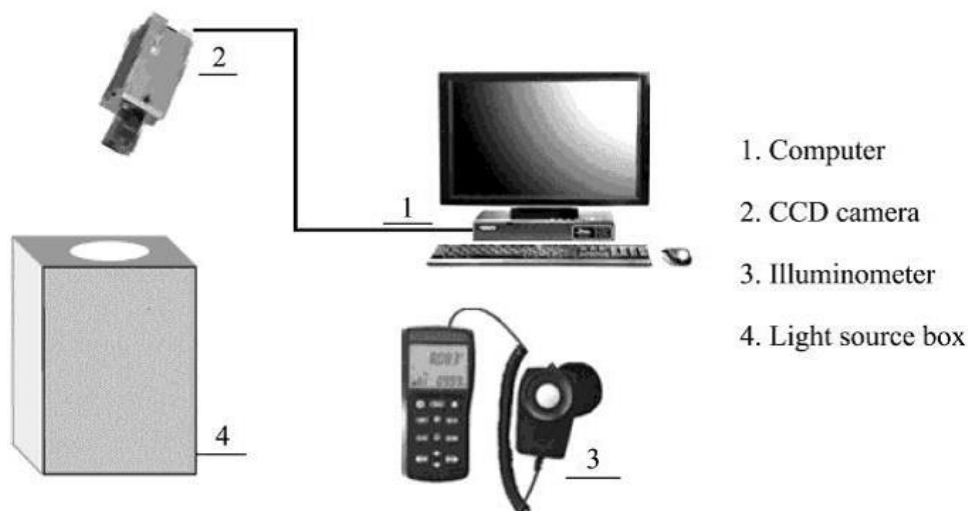
Figure 1. The main components of computer vision system (Tan et al., 2014)
